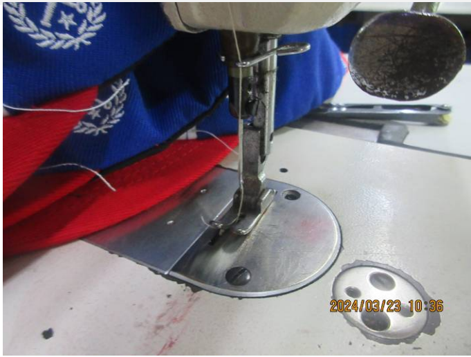
NC-Sewing machine without finger guard.
