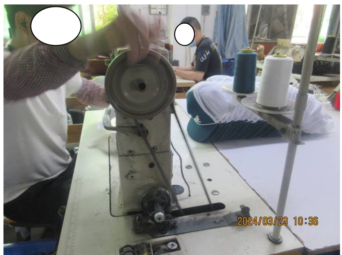
NC- Missing belt guard on sewing machines.
