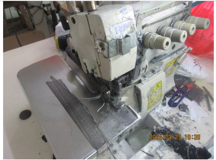
NC-Sewing machine without needle guard.
