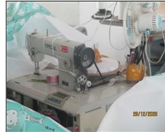
Photo of non-conformity Finding 7.17 No belt guard was installed.JPG
