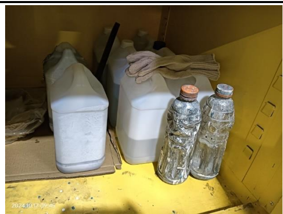
NC-PA7.7-No proper chemical safety labels
