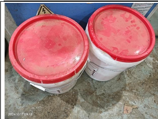
NC-PA7.7-No valid secondary containments
