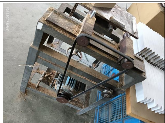
NC-PA7.17-No pulley guard
