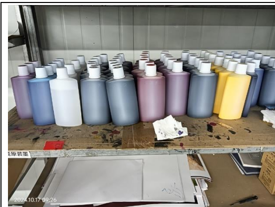
NC-PA7.7-No valid secondary containments and no proper chemical safety labels
