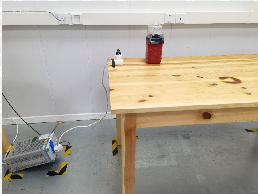
Photograph 1: Set-up for Disturbance Voltage
